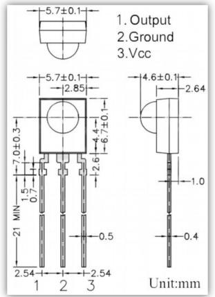
The connection of receiver module is as below:
